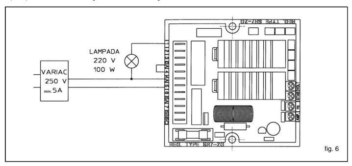
2) Before supplying the circuit with current, turn the "VOLT" and "STAB" potentiometers anticlockwise and the "Hz" and "Amp" potentiometers clockwise to their relevant limits. Position the variac adjustment in correspondence with the minimum value.
