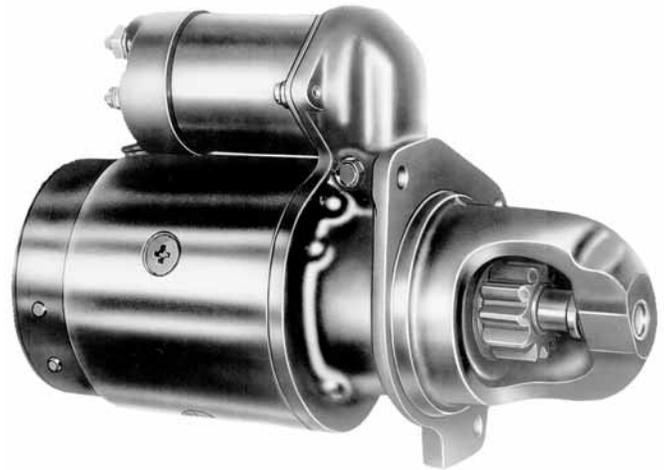
The 10MT is available as "New Service" or a factory remanufactured starter. It is specially designed for high start delivery vehicles. This starter features a design to increase the brush and bushing life. The special field coils effectively limit the top cranking speed, yet still provide adequate cranking speed. The armature coast down time is reduced with the use of brake washer. This unit utilizes a high temperature heavy-duty solenoid.
