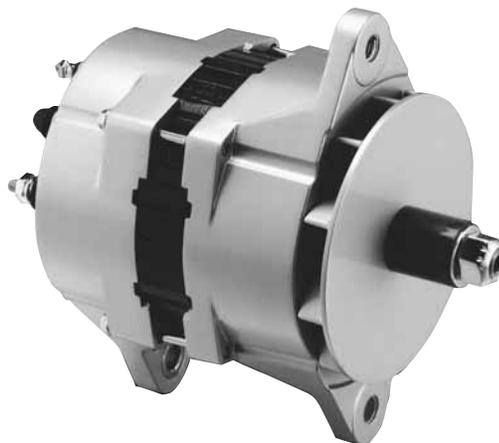
Experience more output and service life for today's mid-range diesels with high electrical load requirements. The brushless design eliminates moving electrical connections. The 23SI offers 70 and 50 Amp outputs in 24 Volt models and up to 130 Amp output in the 12 Volt models, all suitable for most off-highway and medium duty applications.
