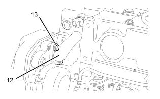
**8.** Install new O-rings onto the bypass tube (12). Apply POWERPART **21820221** Red Rubber Grease to the O-rings. Install the bypass tube (12) into the cylinder head. Install the setscrews (13).
