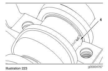
Note: Ensure that the lower bearing shells (3), the upper bearing shells (4), and the appropriate main bearing caps (2) are kept in sets and in the correct sequence for installation.
