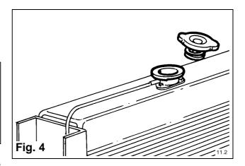
After installation and before the first start remove the radiator cap **Fig. 4** by rotating it anti-clockwise. Fill the cooling system with the required coolant. Should the engine be fitted with water cooled exhaust manifolds then these may need bleeding (see **Workshop Manual Section F7**). Run the engine off-load for one minute to ensure that the system is completely filled, then stop the engine and top up the system to 25 mm (1") below the top of the filter neck then replace the cap.
