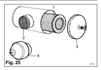
(b) Dust accumulation on the inlet side of the housing is usually caused by leaking gaskets and/or damaged gasket surfaces. If this condition exists, leaking gaskets should be replaced and damaged gasket surfaces should be repaired before placing the unit back into service.
