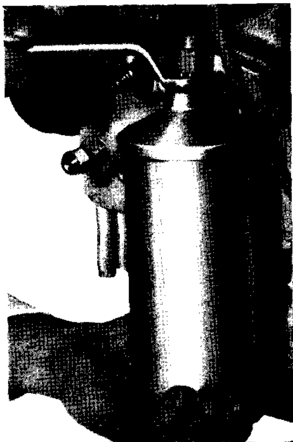
Fig. 17. Unscrewing the Oil Filter Bowl Securing Bolt
